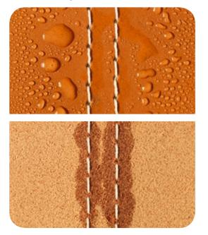
Water stains on the seam when using sewing threads without WR-finish (capillary action/ wicking)
